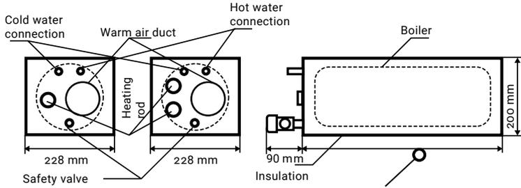
**WITH ONE HEATER    WITH TWO HEATERS**
