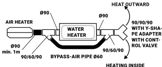
**HIGHLY RECOMMENDED FOR INSTALLATIONS WITH 4KW HEATERS,**
